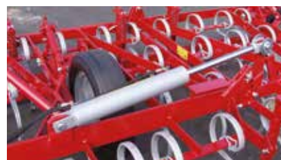
Folding and unfolding with double-acting cylinders.
