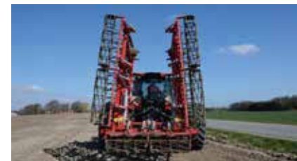
Vertical folding to maximum 3,0 m transport width.
