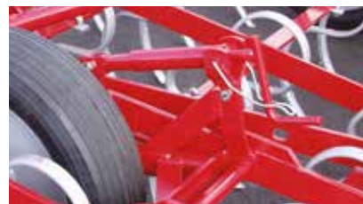
Spindle adjustment with scale.
