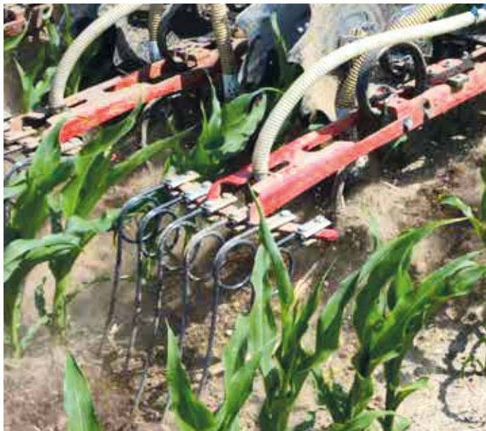
Simple and sturdy rear harrow protecting FS Seeder spreader plates.
