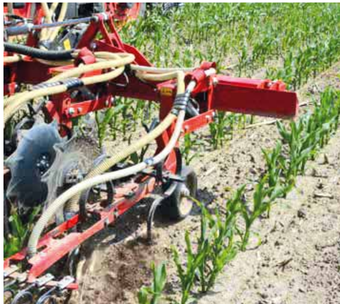
Cleaning sections with genuine Kongskilde tines and shares and rotating plant protection shields for optimum cleaning.
