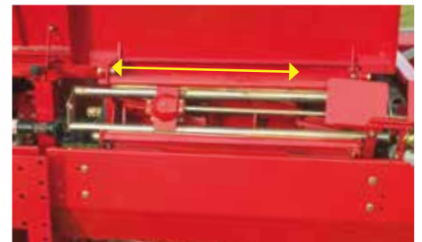
Knife sharpening is very simple. The direction of rotation of the rotor is changed and the dressing stone is pulled back and forth.
