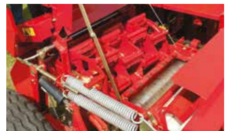
It is very easy to get access to the chopping rotor, simply fold down the chute.
