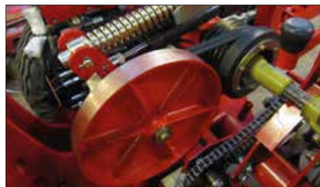
Reverse system is activated from the cabin.
