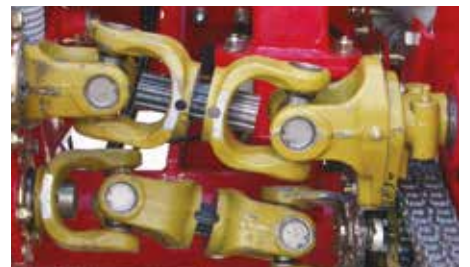
Drive shaft driven feed intake
