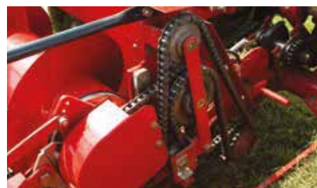
All gears and chains are hardened which gives a considerably longer life.
