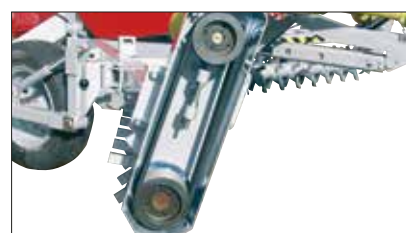
A V-belt pulley powers the stone rakes.
