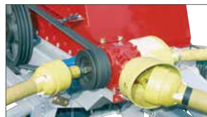
The rotor is powered by a reversing gearbox and a straight V-belt pulley.
