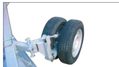
Adjustable double wheels control the depth of the SB 5200 stone rakes.
