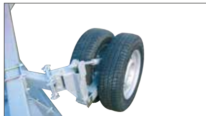
Adjustable double wheels control the depth of the SB 5200 stone rakes.
