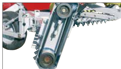
A V-belt pulley powers the stone rakes.
