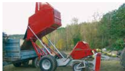
The hopper has a tipping height of 2.3 metre.
