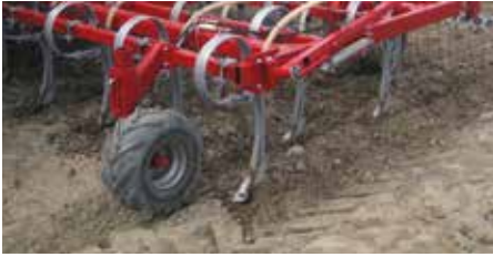
Precise depth control is achieved by the large low flotation tractor pattern tires.
