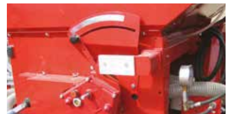
Vario-K stepless transmission.
