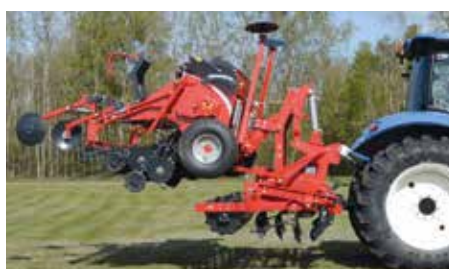
Hydraulic drill linkage for mounting the seed drill on cultivator.
