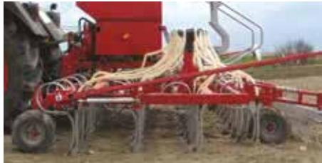
4 rows of tines allows easy passage of field residues.
