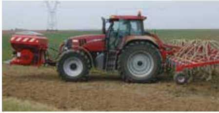
Use of the front hopper gives a good weight distribution.
