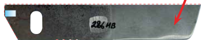
High-strength steel (S650) after the test
