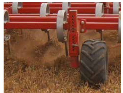
Low pressure wheels ensure precise working depth.
