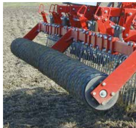
Single FL harrow with semi-pneumatic roller.
