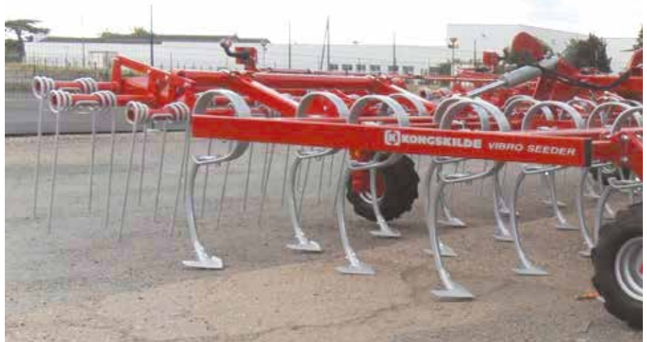
4 rows of teeth facilitate the passage of plant residues.
