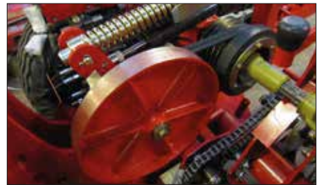
Reverse system is activated from the cabin.
