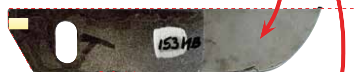
Quality steel (S355) after the test
