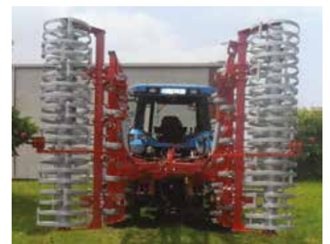
Folding the chassis into two parts allows a transport width of 3 m.
