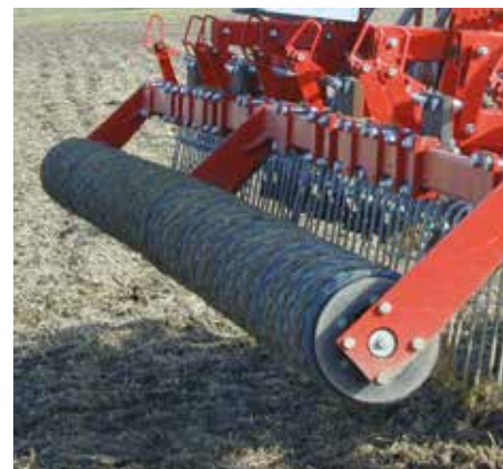
Single FL harrow with semi-pneumatic roller.
