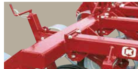
VF 4200 / 4300 / 4000 Rubber wheel 24 x 8.00 - 14.5 with spindle adjustment.
