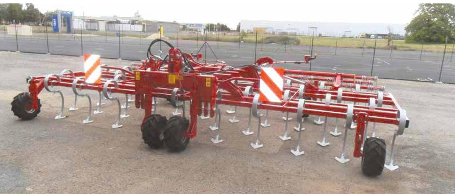
Single FL harrow with semi-pneumatic roller.
