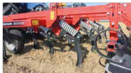
C-shaped Delta Flex tine.
