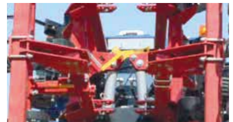
Automatic hydraulic wing lock system.
