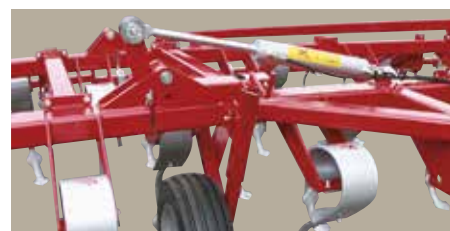
VF 4200 / 4300 / 4000 Folding with double acting cylinders.
