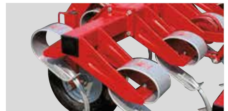
VF 2000 Bolted on side extensions.
