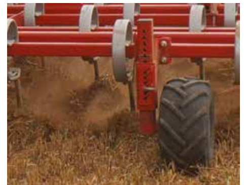
Low pressure wheels ensure precise working depth.
