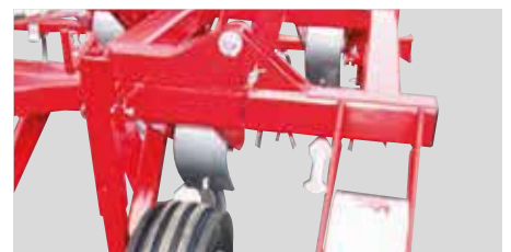
VF 4200 / 4300 / 4000 Rubber wheel 6.00 x 12" with spindle adjustment.
